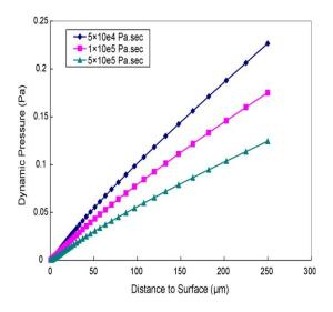
Fig.5 Dynamic pressure distribution normal to specimen surface with different media viscosity for 5MPa extrusion pressure.
