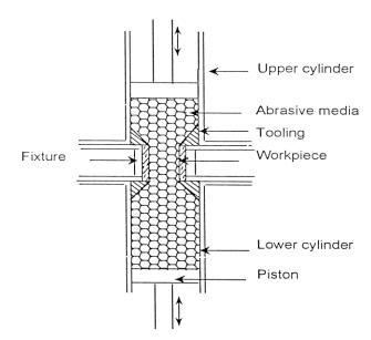
Fig.1: Schematic showing AFM process
