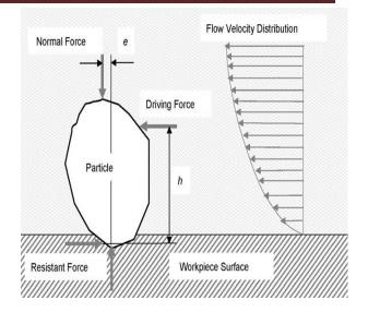
**Fig.7** Schematic of force analysis acted on a particle in AFM suspension media.
