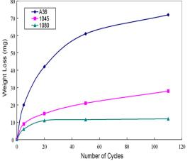
Fig.9 Relation of the number of cycles to wear weight losses for AISI 1045, 1080 and A36 steel.
