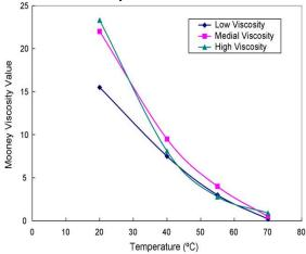
**Fig .4.** Variation of Mooney viscosity with temperature for three types of suspensions. *L. Fang et al*
