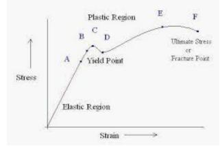
Fig.2: Stress vs strain diagram
